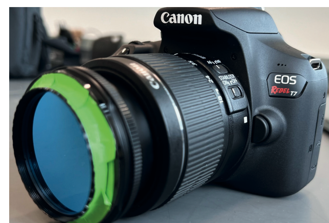
IMAGE 4: MODIFIED CANON REBEL T7 AFFIXED WITH BAADER UV BANDPASS FILTER
