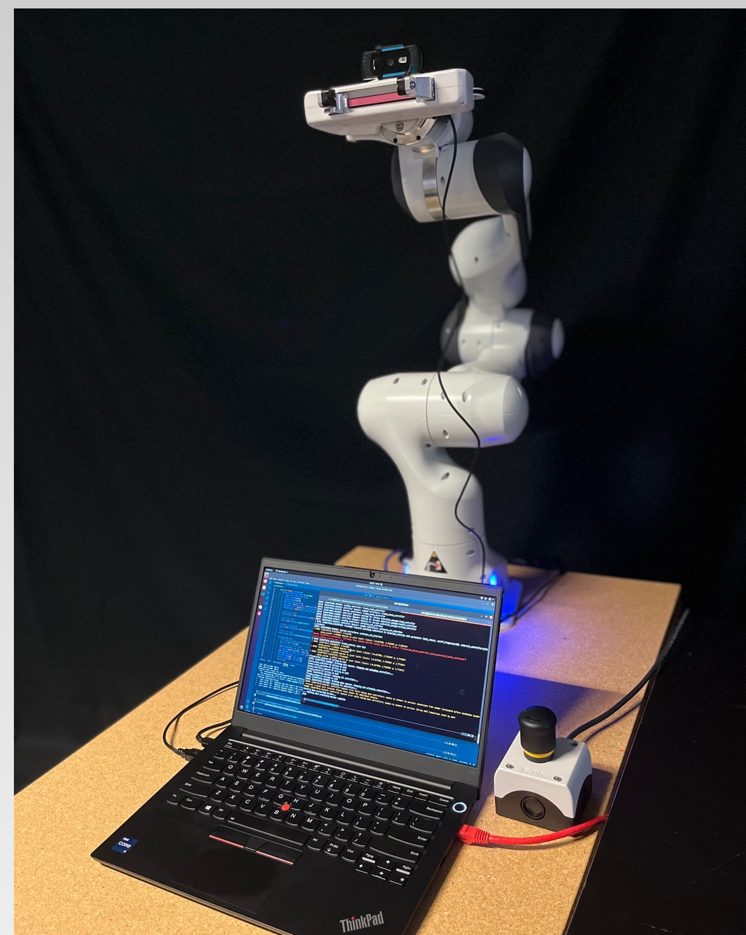
Figure 2: Project Set-up. A Franka Emika robotic arm with webcam mounted at the end-effector (gripper). The webcam is connected via USB to the laptop, and the laptop is connected back to the arm via an ethernet cable.
