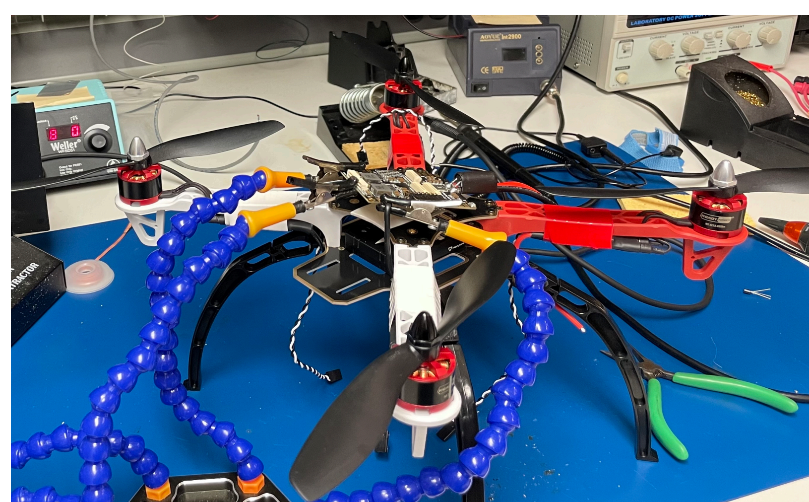
Soldering the engine speed controller power leads to the power distribution board
