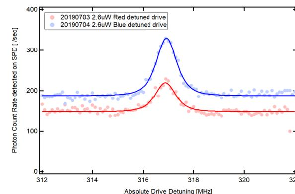
• **Figure 5:** Data collected shows the amount of red and blue shifted photons observed exiting the optical cavity. Classify the amounts would be the same. The difference can be explained by the laws of quantum mechanics and energy having to exist at discrete values. SPD  $\equiv$  Single Photon Detector
