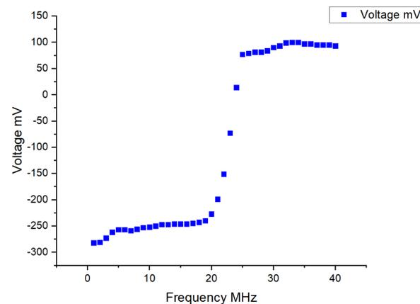
• **Figure 3:** Error signal output voltage dependent on an input frequency from a signal generator. Any change in the beat frequency corresponds to a change in voltage in the error signal. It is important to have a steep slope around the zero-voltage point because this will correspond to a strong response in the error signal and an effective feedback loop keeping the frequencies of the lasers locked in the correct position.
