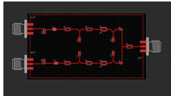
• **Figure 2:** Computer drawing of frequency to voltage converter (FTV) used to create printed circuit board with surface mount devices. The circuit contains two separate branches that rectify the AC sine wave into both a positive and negative voltage and then adds them together. This DC output is then used as the error signal for a feedback control loop.
