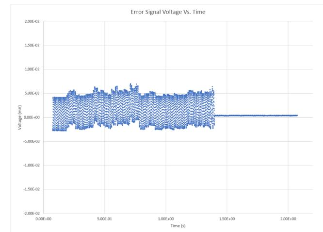
• **Figure 6:** This plot shows when the PID was engaged to lock. The error signal goes from an oscillating voltage that is dependent on the frequency of the input signal to a constant voltage around 0 V.
