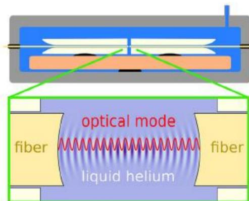
• **Figure 1:** Optical Cavity containing volume of super fluid liquid helium. Photons tuned to a specific frequency enter the cavity and interact with the superfluid liquid helium. The photons either give energy to the helium or take energy from it. The photons then exit the cavity and are then observed.
