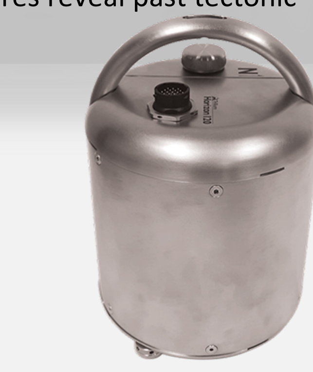
Above: IGU-16HR-3C nodal sensor at site 35 in Charlemont, MA. This sensor can record most large earthquakes anywhere in the world
