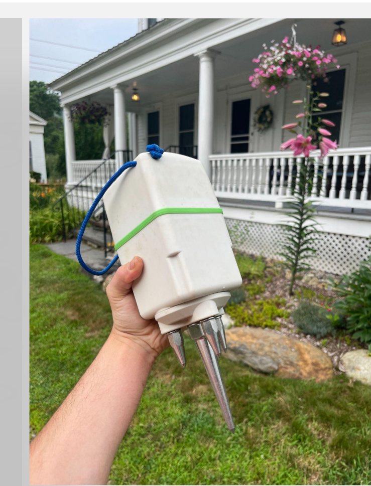
Above: IGU-16HR-3C nodal sensor at site 35 in Charlemont, MA. This sensor can record most large earthquakes anywhere in the world
